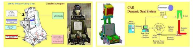
H8.1 <u>Seat pressure pad</u>. This gives an effective cue of seat pressure under G, particularly for the lower G values before G-suit onset. I have also flown a simulator with multiple seat pads with different inputs, but these are complex, expensive, can give confusing cues, and are not recommended.
